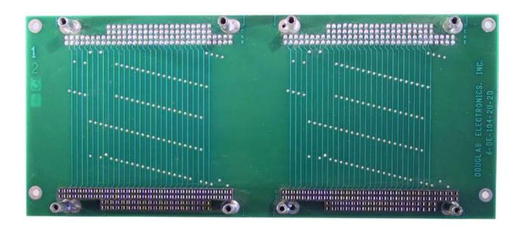
The 6-DE-104-2U-2D board allows four PC/104 stacks to be joined. Two side-by-side stacks are on top of the board and two side-by-side stacks are on the bottom of the board. Each of the four stacks has the solder side of the board facing the 6-DE-104-2U-2D board.
