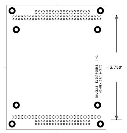
The 6C-DE-104/16-3.75S board allows two stacks of PC/104 boards to be joined with the solder side of both stacks facing the 6C-DE-104/16-3.75S board. An alternate is to use the 6C-DE-104/16-3.75P board and have the component side of each stack facing the 6C-DE-104/16-3.75P board.
