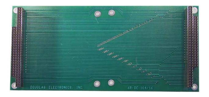
The 6R-DE-104/16 board supports two PC/104 with the PC/104 connectors at opposite ends of the board. The board is normally supplied with Sockets only.
