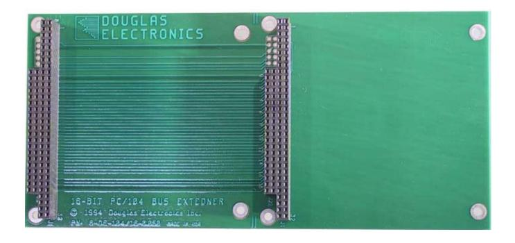
The board is 3.600" x 7.600" representing two standard PC/104 footprints with 0.050" clearance between boards. The boards are available with stack-through connectors, Pins only or sockets only. This board is exactly the same as the 6-DE-104/16 (W18) except that it is 0.200" shorter allowing only 0.050" between the two PC/104 boards.
