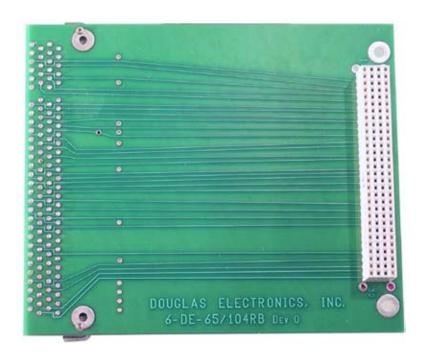
The 6-DE-65/104RB is designed to place a PCI board on the bottom of a PC/104Plus stack. The board has a female 120 pin PC/104Plus connector and a PCI slot that is below the 6-DE-65/104RB board. This board must be the bottom board in a stack.
