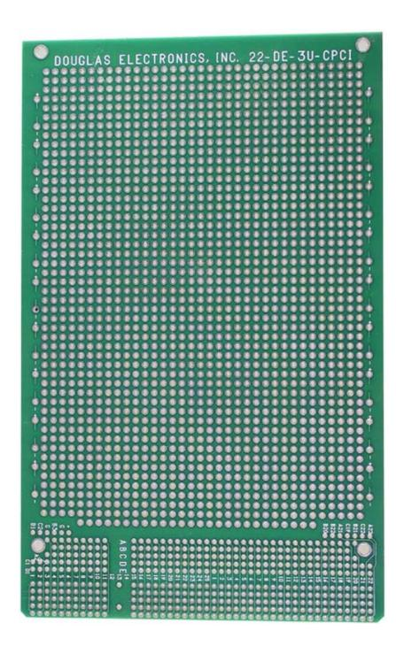
The 22-DE-3U-CPCI 65 is a breadboard for creating your own cPCI interface boards. The entire surface is filled with pads on 0.100" centers. Each pad is 0.070" diameter with a 0.038" plated-through hole. The component side has a Ground-plane and the solder side has a Vcc plane.
