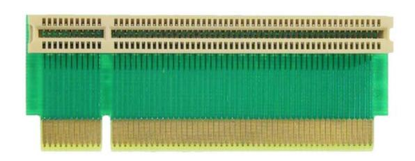
The 6-DE-65RR boards provide a right angle connector to allow a PCI board to be mounted in a PCI bus, but not take the normal height required. The board is available in several configurations. See the attached drawing to be sure you are selecting the correct one for your application.
