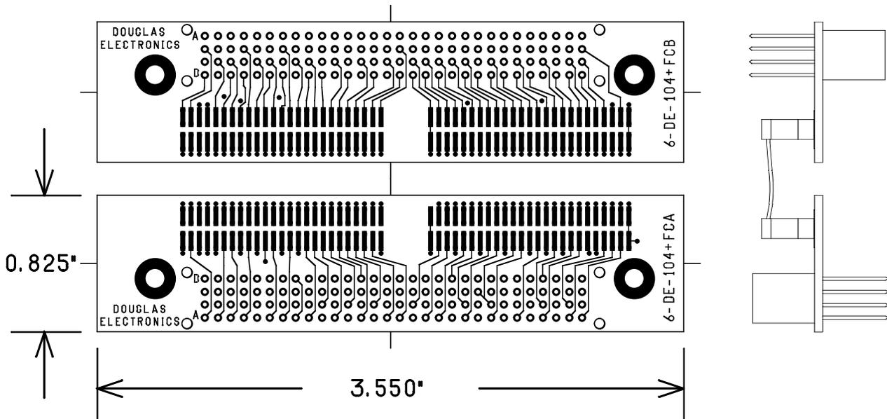
The 6-DE-104+-FCA/B is a flat cable extender for the PC/104 bus. Flat cable is not good for carrying high-speed signals and we do not recommend this product; however, customers have wanted it and we have made it available. Clearly, the shorter the cable the more likely you will have success.
