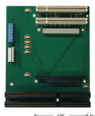
The BX-DE-104+-263-265 board provides a location for a PC/104Plus board (or stack), two PCI boards and two ISA boards. Power connections may be made at either of the two power connectors
