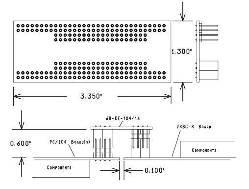
The 6B-DE-104/16 board can be use to minimize the height of a PC/104 stack by splitting them into two stacks. When the board is used, one of the stacks has the component side up, the other stack has the component side down. The PC/104 connectors of the two stacks are close to each other. The board is normally supplied with a male connector on one side and a female connector on the other side. Optionally, one or both of those two may be replaced by a pass-through connectors.
