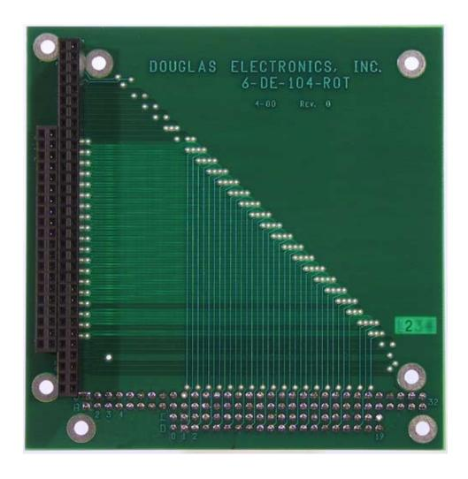
The 6-DE-104-ROT board allows a PC/104 stack (not PC/104*Plus*) to be rotated. The rotation can be either clockwise or counter-clockwise. The board is normally supplied with pins only at one location and sockets only at the other location.
