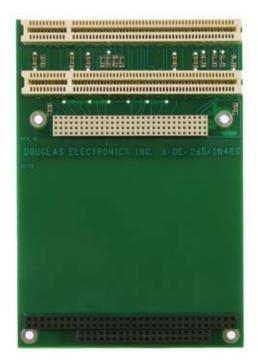
The 6-DE-265/104RS board is identical to the 6-DE-65/104RS (W-06) board except that this board provides two PCI slots. The slots are behind the PC/104 stack. The board may be placed low in the stack so that the height of the PCI board is not all added to the height of the total assembly. The two PCI slots a 0 and 1.
