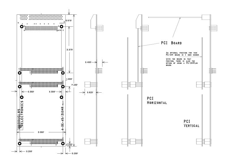
The 6-DE-65/3104R boards provide for a PCI board mounted parallel to the other boards in the stack, and for two PC/104 (non plus) stacks. The PC/104 stacks are offset from the PC/104 bottom stack by 1" which allows the PCI board to lay flat and avoid conflict with the PC/104 stacks. The PC/104 connectors are elevated from the board by 0.400".
