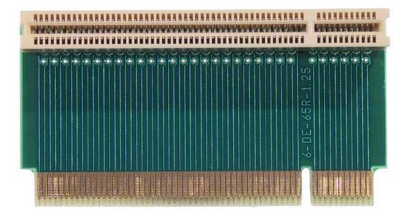
The 6-DE-65R boards provide a right angle connector to allow a PCI board to be mounted in a PCI bus, but not take the normal height required. The board is available in several configurations. See the attached drawing to be sure you are selecting the correct one for your application.
