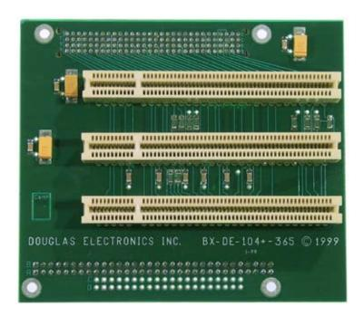
The BX-DE-104+-365 board provides sockets for up to three PCI boards on the top of a PC/104Plus stack. This board must be the top board on the stack.
