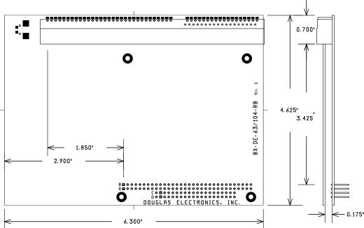
This board is available in three other versions - the only difference being the relative location between the PC/104 connector and the ISA connector.
