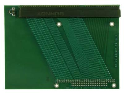
The BX-DE-63/104-RB board allows a single ISA board to be used in a PC/104 stack with the ISA board parallel to the individual PC/104 boards.
