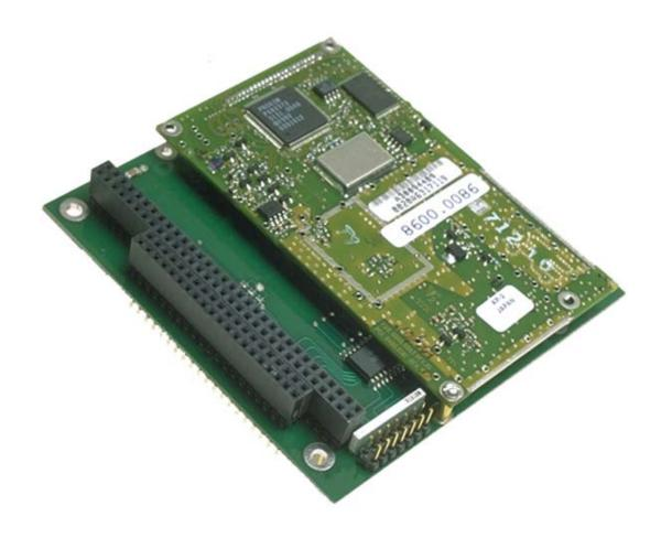
The 6-DE-PROX/104 interfaces the Proxim RangeLan2/OEM Wireless LAN Board to a PC/104 bus. Address and interrupt requests may be set by the user (some soldering is required to change the interrupt request).
