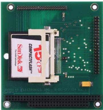
The 6-DE-CF/104 board interfaces a SanDisk CompactFlash (or equivalent) with an Ampro CoreModule/3SXi or /4DXi, or an Ampro Little Board/486i or /P5i (or equivalent boards). A flat cable is required (but not included) to complete the connection from the disk to the associated board.
