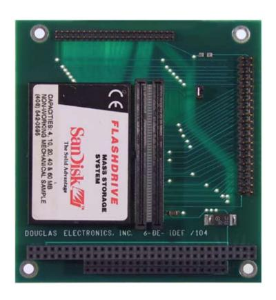
The 6-DE-IDEF/104 board interfaces a 1.3" IDE Flash Disk (such as the IDE 2000 series from M-Systems) with an Ampro CoreModule/3SXi or /4DXi. or an Ampro Little Board/486i or /P5i (or equivalent boards). A flat cable is required (but not included) to complete the connection from the disk to the associated board.
