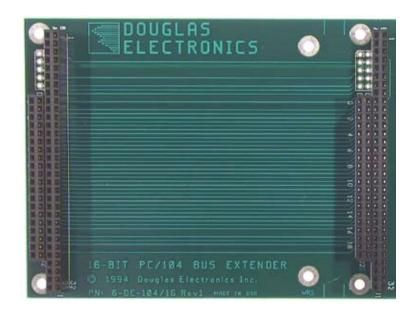
The 6-DE-104/16-4750L-P is equivalent to the 6-DE-104/16 board (W-18), except that the overall board length is altered to 4.75 +/- .02 inches.
