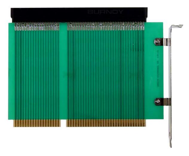
The 6-DE-63 is an extender for the ISA bus that allows one ISA board to be lifted above the others for in-circuit testing. The circuit board measures 6.200" x 4.200". The extender supports 8-bit or 16-bit operation.
