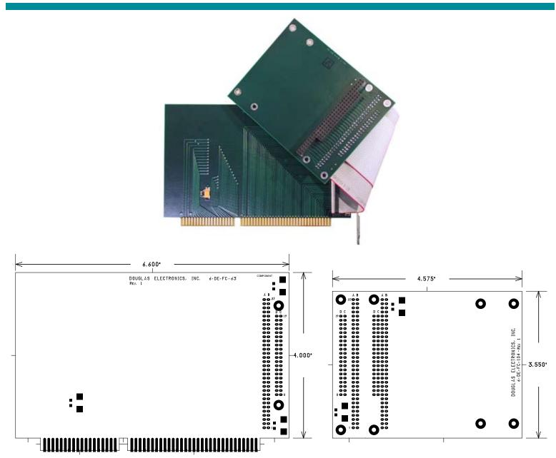
The 6-DE-FC-63/104 board pair allows supporting a PC/104 stack – via flat cable from an ISA bus. It is designed to allow the PC/104 stack to be on the back, outside of a standard ISA box.
