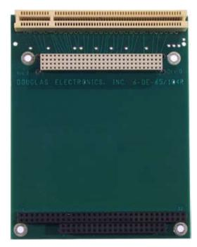
The 6-DE-65/104RS board supports a single PCI board from a PC/104Plus stack. The RS model positions the PCI slot perpendicular to the PC/104 stack. The 6-DE-265/104RS (W-45)board is also available that supports two PCI boards.
