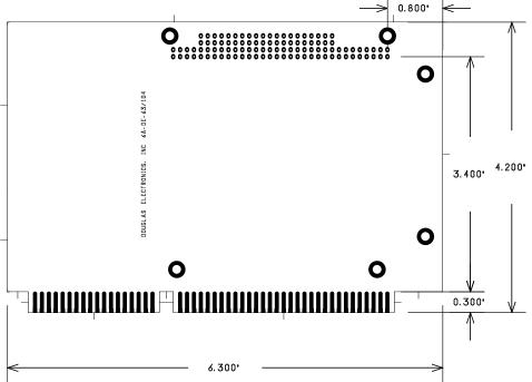
The 6A-DE-63/104 allows 8 or 16-bit PC/104 modules to be used completely inside an ISA box. When installed, the top edge of the PC/104 module is flush with the top of the 6A-DE-63/104 board. The board is 6.300" x 4.200". The PC/104 socket is on the component side of the 6A-DE-63/104. Plugging in a PC/104 board puts the solder side of the PC/104 against the component side of the 6A-DE-63/104.
